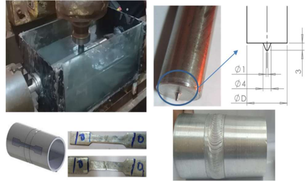
Fig. 1. (a) UFSW of AA 6061 pipes using EG-FSW-M1 equipment. (b) Conical friction stir welding tool (c) Test specimens fabricated with ASTM D3039 standards. (d) Underwater friction stir weld images of Al 6061 pipe
